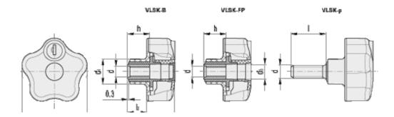
$$\begin{array}{ll} D & = 63 \\ d1 & = 23 \\ d \ 6H = M6 \\ h & = 18 \\ I & = \\ L & = 44 \end{array}$$
